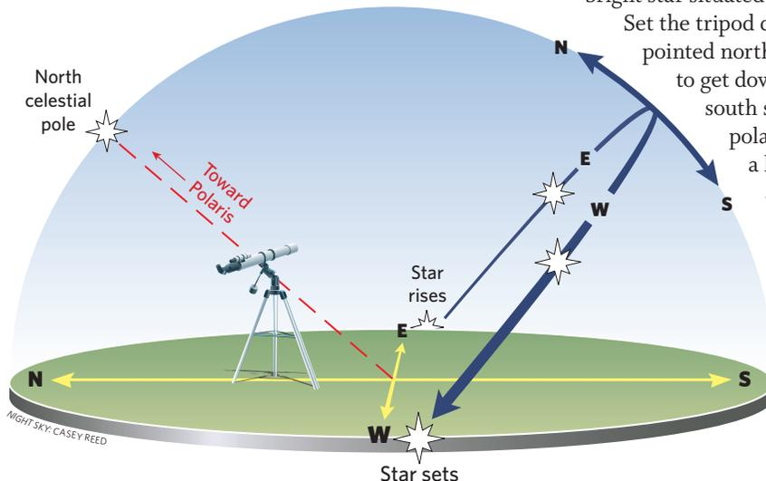
**FRAME OF REFERENCE:** The essence of polar alignment is simply ensuring that your mount’s polar axis (also known as the *right-ascension axis*) is aimed at the north celestial pole, located near the star Polaris.
